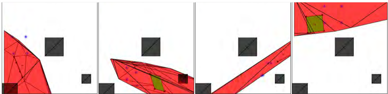
(c) Projection (red) of the convex obstacle-free polytope \mathcal{P} onto the 2D top view at approximately the same time instances of the snapshots. The projection can overlap with obstacles that are not in the field of view of the robots. The projection of the optimized formation is shown in green and the convex hull \mathcal{C} of the robot positions at the time of computation with blue stars (recall that the optimized formation is only recomputed every 2 seconds). In two frames the projection of the optimized formation has negligible size and is shown by a line.
