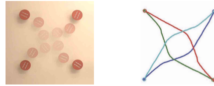
Fig. 11. Experiment with four e-puck robots exchanging antipodal positions. Time-lapse and trajectories. Trajectories are smooth and collision-free.
