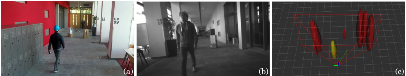
Fig. 7: Results of the experiment Scenario 2. The MAV is flying in a corridor while avoiding static and moving obstacles. (a) A snapshot during the experiment. (b) An on-board grayscale image captured in the experiment and (c) visualization of the corresponding obstacle detection and trajectory planning results.
