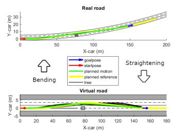
Fig. 1: The proposed motion planning method applied during high-speed driving on a curved highway.
