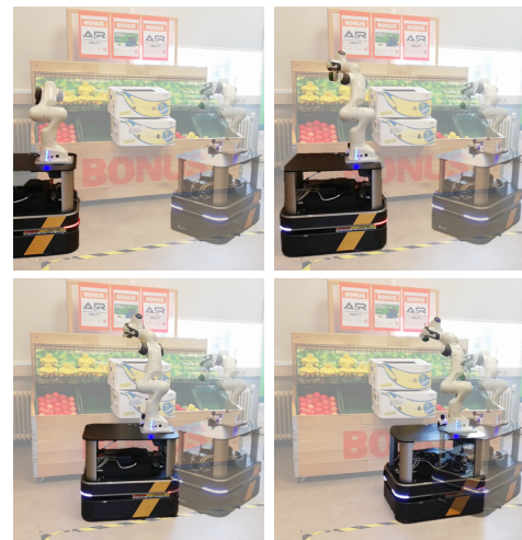
Fig. 10: Trajectory in mock-up store avoiding obstacles, goal configuration in light grey.
