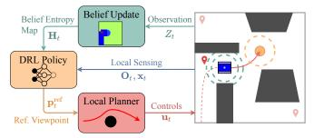
Fig. 1: Conceptual overview of the proposed informative trajectory planning framework. A DRL policy recommends a viewpoint reference to a local planner, based on the robot's current belief about the environment, and local sensory information. The local planner generates a feasible trajectory and executes control commands, leading the robot (depicted in blue on the right-hand side) to reduce the uncertainty about the environment.
