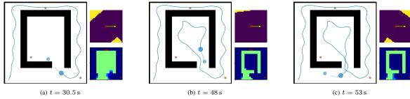
Fig. 5: Trained policy behavior in a *structured* environment of higher complexity than in training, with three timesteps of an episode displayed. The three snapshots show that the robot is effectively guided into and out of a room-like structure, without visiting areas twice. The setup of the figures is as described in Fig. 4.
